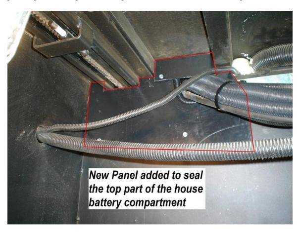
Most of the air holes in the compartment were sealed with either foam or plastic panels leaving enough openings for battery gas venting. IMO Tiffin leaves to much open area around the batteries creating a mess which is hard to keep clean and contributes to a shortened life of the batteries.
