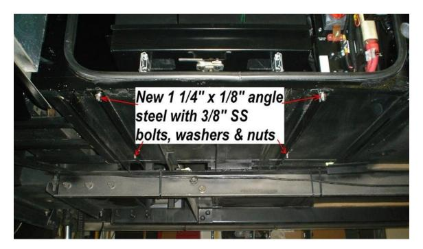
In a soon to be made modification, six new HOUSE batteries, 648 Ahr will be installed along with a battery tray in the old LP tank compartment located in the passenger side front compartment. The new HOUSE battery bank along with the six OEM battery bank will when completed consist of twelve Interstate wet-cell batteries with a combined 1296 Ahr rating.
