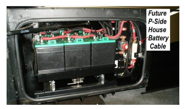
The new P - Side cable is installed near the 300 Amp fuse ready to be connected after the six new batteries and tray are installed.
