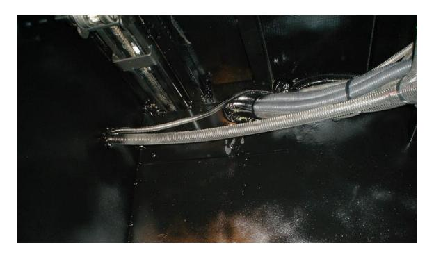
The above picture was taken after sealing and painting. I took this opportunity to install additional house battery cabling between this D - Side HOUSE Battery Compartment and the soon to be P - Side HOUSE Battery Compartment front (the old LP tank) compartment.
