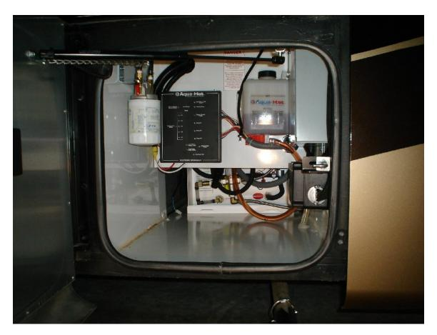
The Aqua-Hot compartment on the driver's side has been made user friendly, components have been relocated making them more accessible for servicing. Components in this compartment include: a Progressive Industries EMS-HW50C, a Tiffin 3rd Generation Transfer Switch, and the Aqua-Hot's coolant reservoir, Control Panel, and Fuel Filter.
