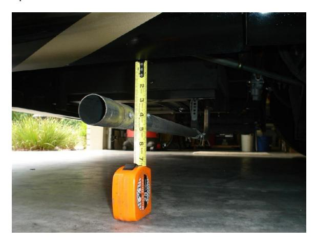
I suggest everyone should check those two generator tail pipe bolts to ensure they are tight. Tiffin installed the two bolts on my generator without using lock washers, which I highly recommend be installed if not already installed. Comparing the above and below pictures shows the amount of generator tail pipe that was cut off in order to increase the generator exhaust pipes road clearance.
