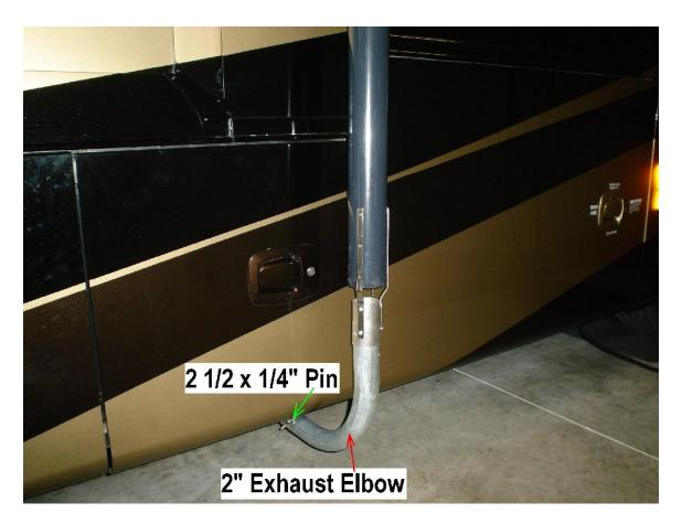
One short exhaust pipe extension with a 2 1/4 " ID on one end and a 2 1/4 " OD on the opposite end was purchased from the local Advance Auto Parts store. The stock 1 1/2 " exhaust elbow was removed from the lower section to be replaced with a 2 " ID EMT elbow. 6 - 3/16 " x 1/4 " pop rivets were used in re-mounting the three brackets to the exhaust pipe extension, Pop rivets and EMT elbow were purchased from the local Lowe's store.
