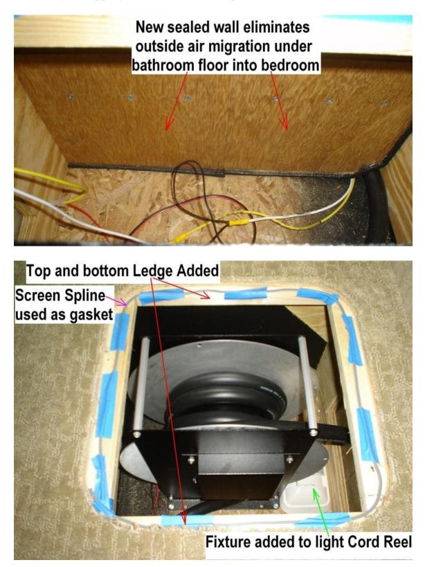
Both top and bottom ledges around the cord reel access hole were added along with the screen spline to act as a seal between the closet and the cord reel compaartment. Now when the closet floor cover is screwed in place the Shore Power Cord Reel Compartment is isolated from the rest of the coach. No more dirt, dust or pollen through the cord access into the coach.
