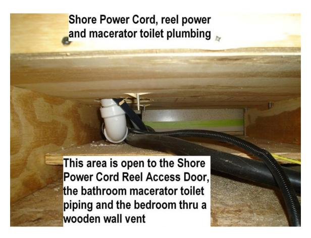
The above area is the camera view taken inside the cord reel compartment looking under the raised bathroom floor.
