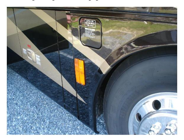
When the driving lights are turned ON, we have two additional side lights to shine our location, just in case our small vehicle cannot be seen. Also when the turn signals are active a driver in the adjacent lane will have additional warning that I desire to move over into that lane.
