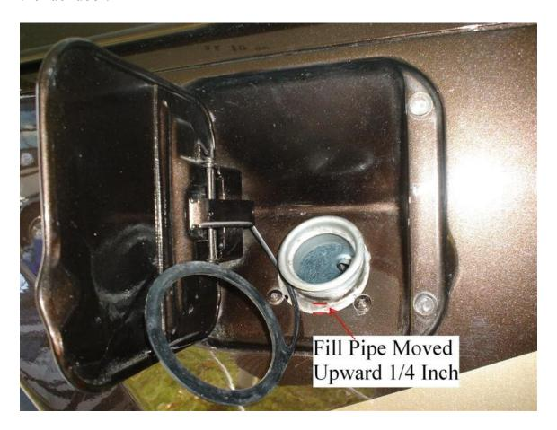
I removed the two screws holding the fill pipe in the fuel fill box. After the fill pipe had been moved out of the way, a round file was used to remove the necessary amount of fiberglass to allow the fill pipe to be moved upward
