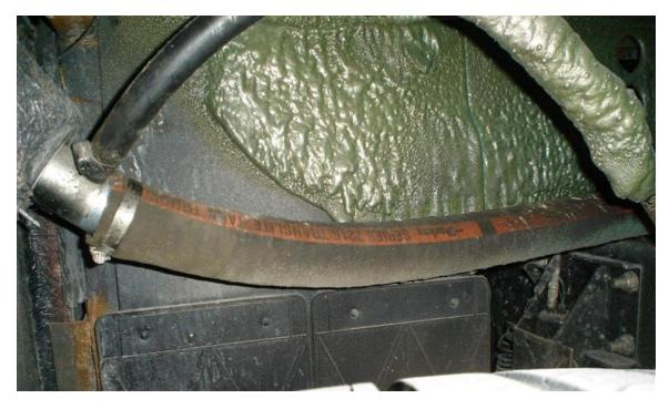
I decided to modify the way both fuel fill hoses were mounted. Alas the first attempt did not help at all. I had been told to loosen the hose clamps on both ends of the hose, then turn the hose (rotate the low part of the hose to the top) then re-tighten the hose clamps. It did not take long for me to realize that at best this was a short term fix, as when the hose bowed again due to gravity the bow/sag would be back at the bottom.
