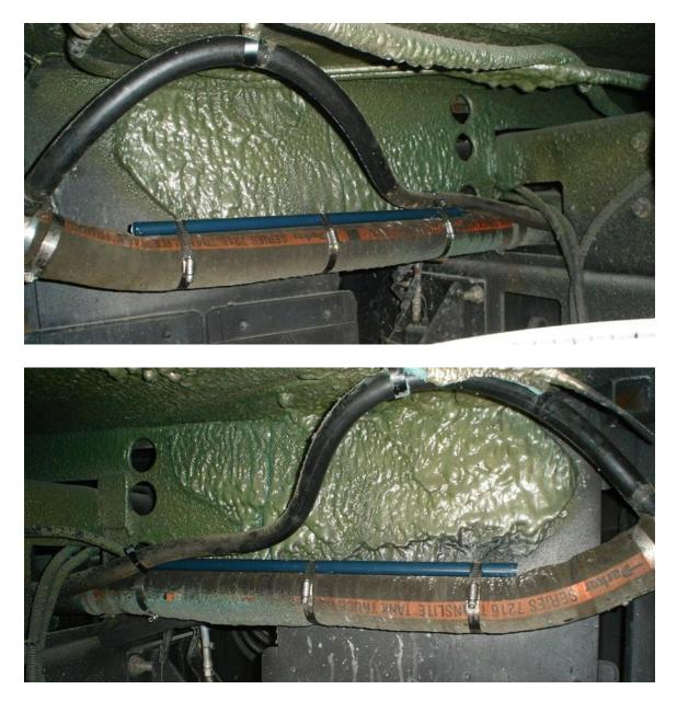
The above DS fuel fill modification shows the downward slope of the fill pipe between the fuel fill and the fuel tank and it also shows the tank vent hose does not have a low point in which fuel can collect which then shuts OFF the fuel nozzle when a fuel bubble is expelled.
