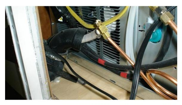
The RR Ice Maker Water Line is installed inside the below 1 1/2 inch ABS pipe by Tiffin. The pipe is the only protection again freezing temperatures.
