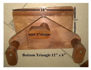
The computer mounting surface is constructed from ½ plywood cut 10 inches long by 7 inches wide. To enable the mounting surface to turn one 1½ inch wood screw was centered in the surface and screwed into the triangular mount. A flat washer was installed between the two wood surfaces to act as a bearing allowing the top surface to rotate, to make rotation stiffer the
