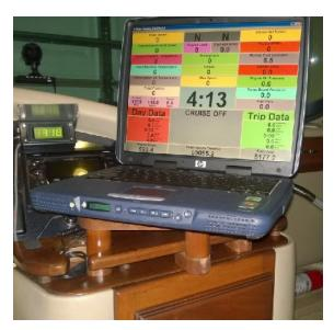
The feet were installed on the dowels by using 2 inch long wood screws. Velcro strips were installed on the top surface and mating Velcro strips were installed on the bottom of the computer.
