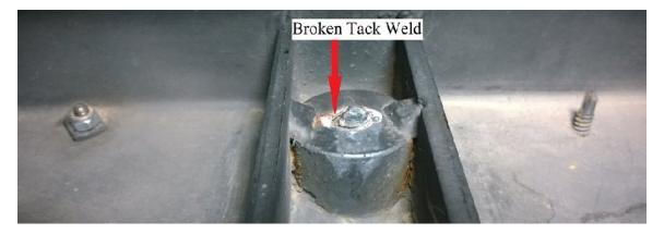
The problem many owners have or will have, the tack weld breaks as shown above when that happens the shoulder bolt will slowly work itself loose, when the bolt works loose a gap develops as shown below, as the gap develops the operation get nosier then normal if not corrected parts break.
