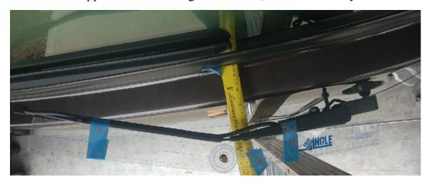
As shown above the windshield is recessed 2 ½ inches this wiper arm was not designed to be used with a recessed windshield. One quick method to correct the problem is to insert a 15 ° bend in the wiper arm as seen below. While the arm is strong it can be bent using just your hands. The bend needs to be rechecked over time as the arm will lose the 15 ° bend over time.
