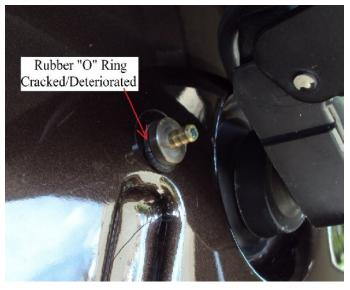
As seen in the photo the wiper arm hose cracked requiring the hose to be replaced. Tiffin sales the wiper arm hose in four foot sections, on our 2010 Allegro Bus the four foot section is just barely long enough to replace both hoses using one kit. The hose reaches from the brass hose attachment mounted in the front cap to the spray nozzles mounted on the wiper arm.
