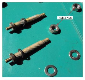
The spray hose brass connectors are inserted thru the front cap a washer is placed over the brass connector on the inside of the front cap then a 14 MM nut is installed.
