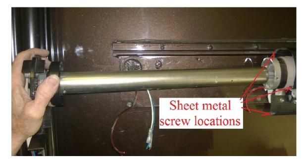
The above photo shows the assembly reassembled and being reinserted into the awning tube. Keep in mind the lower LEGS of the Jumping Jack straddle the rolled portion of the tube which is used to slide/insert a drop down shade.
