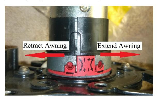
After the repair the **RETRACT** awning **STOP** setting required turning **SEVEN FULL REVOLUTIONS** in the – direction before the motor would **STOP** where it needed to **STOP** without being stalled to a **STOP**. Each time the awning motor retracted and **STALLED** to a **STOP** contributed toward the wringing apart of the awning motor shaft.
