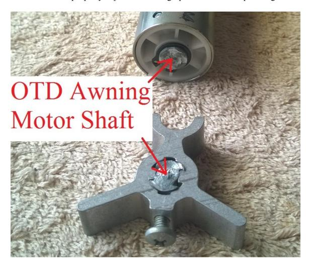
The below photo shows the way the motor shaft looks when it is not damaged. The Philips head set screw keeps the Jumping Jack in place, my term for the aluminum figure which appears to be a Jumping Jack with a Phillips screw head.
