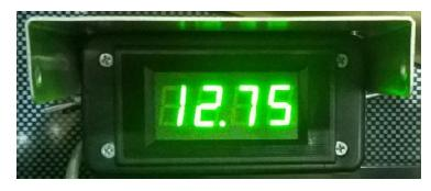
The dash mounted meter shown on the left displays either the CHASSIS battery voltage OR HOUSE battery voltage depending on the position of the switch on the left side of the meter. It is
