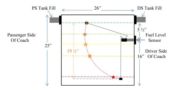
RED dashed line is the ARC of the Fuel Sensor Float
