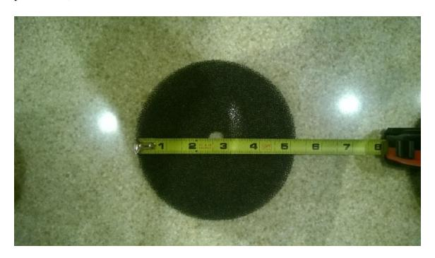
As seen in the above photo, the diameter of the foam filter is 5 1/4" the diameter of the hole in the center is 1/2". The filter material is 1/4" thick. I find exchanging the filters every few weeks by using the second set of filters easier. Then the filter are washed, allowed to air dry then stored in a zip lock bag until next time. IMO, rotating the filters in this manner is easier than just having one set to remove, clean, dry and re-install.
