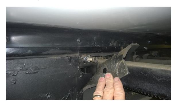
I'm not sure what caused the forward stop bolt nut to fracture? However this is just one more item I'll need to keep an eye on.
