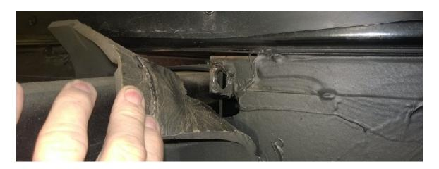
As you can see in the above photo, the nut tack welded to the slide frame fractured allowing the bolt and one nut to fall out of the hole, finally resting on the ledge under the slide mechanism.
