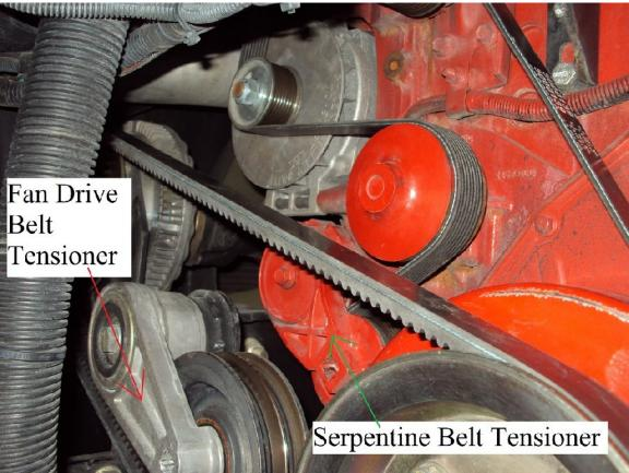
The  $\frac{1}{2}$ " drive bar was again used to release the tension on the belt tensioner once the tension has been removed the belt can be slid off a pulley I used the
