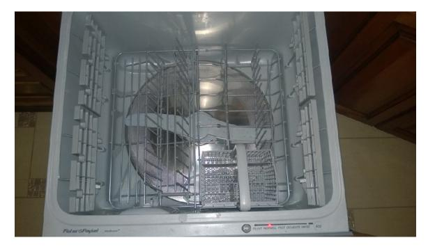
Looking into the open dishwasher drawer, the basket needs to be removed to begin maintenance. IMO, the easiest method to remove the basket is to grab the rear side of the basket with both hands, lifting up then lift the left rear tilting the basket to slip it past the rinse basket on the front of the drawer.
