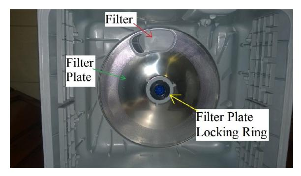
After the filter plate has been removed the rotor is accessible.
