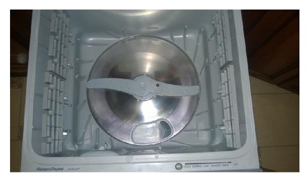
Once the basket is clear the spray arm can be removed allowing access to the filter plate locking ring. Next rotate the locking ring counter clock wise 1/8 turn to unlock the filter plate then lift it out allowing access to the rotor.
