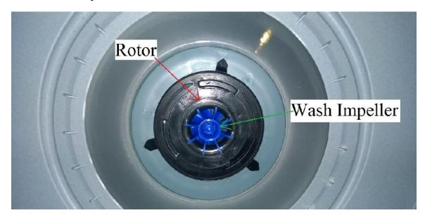
In the case of our unit, the rotor had seized and would not rotate due to some DRIED leftover debris from previous wash cycles. Removing the rotor is a simple counter clockwise turn of the black plate, than you can lift the rotor out of the depression that is part of the motor housing.
