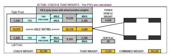
Part 3, is the COMPUTED COACH, TOAD, HITCH & TOW BAR LOAD LIMITS. Again if the coach has three axles you would continue to use this 8 wheel sheet. If the coach has two axles click on the 6 wheels sheet. In this part there are THREE Gray cells that are not LOCKED. As they are unlocked you can enter the date of the weighing, your coach information and your toad information.
