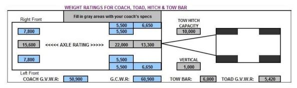
Part 2, is the ACTUAL COACH & TOAD WEIGHTS of each wheel position, in this case six wheel positions, plus the towed vehicle weight and the vertical weight of the tow bar. The EIGHT cells are not LOCKED. Again as they are unlocked you can enter the actual weights of the six wheel positions, the actual weight of the towed vehicle and the actual weight of the tow bar.
