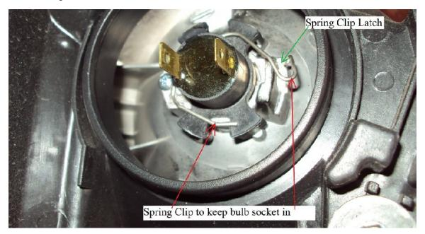
The spring clip is unlatched by depressing the clip where I noted "Spring Clip Latch" in the above photo then moving the clip to the side enough for the clip to bypass the fixture, then you can swing the clip to the opposite side releasing the socket, as shown in the photo below. Make sure to hold your finger on the back of the bulb socket to prevent the bulb socket from falling once the clip has been unlatched.
