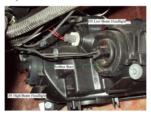
Above is a photo of the DS (driver side) of our Allegro Bus headlight fixture. As seen above I noted the low beam and high beam wiring harnesses. I began this bulb replacement by removing the two wire low beam wiring harness by just pulling straight out so it could slip off the two pins.
