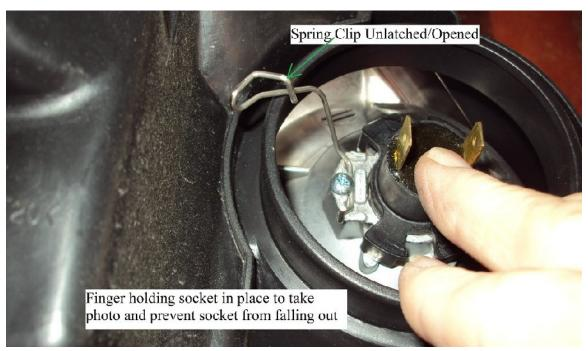
After removing the bulb socket the old bulb can be pulled out of the socket then a new bulb may be pushed back into the socket.
