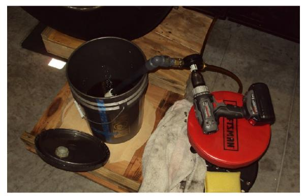
I am a lazy person so I use clear tubing and drill pump to pump oil from the bucket into the differential. The blue tape on the side of the bucket is marked to show me how much oil is in the bucket and when to stop pumping. At the 14.5 quart point the oil began flowing out of the top differential plug hole.
