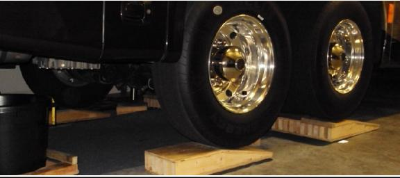
After working the coach high enough to safely work under to drain the differential, the top differential fill plug is removed. After positioning the drain bucket the bottom drain plug is removed to drain the oil. The magnetic center of the drain plug needs to be cleaned to remove metal dust and filings before the plug is re-inserted.
