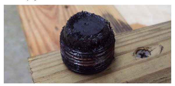
After the plug has been cleaned and the metal removed it is re-inserted into the bottom of the coach differential.
