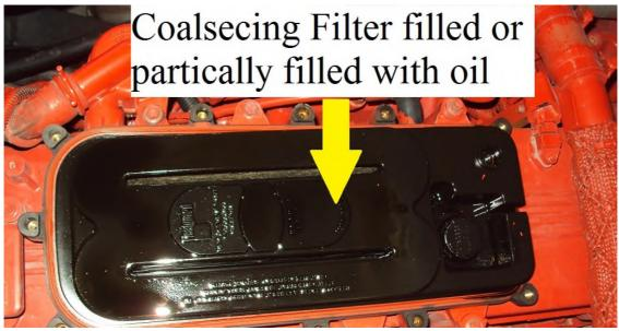
After the 11 bolts have been loosened the plastic cover is easily removed from the top of the engine exposing the old coalescing filter.
