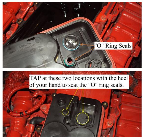
After the cover has been set in place and the "O" rings have been set using the heel of your hand, each of the 11 bolts are started by hand. The cover is
