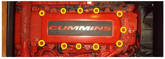
BEFORE removing the cover, clean the area around the filter cover making sure dirt, grease or other debris is not allowed to get into the filter's cavity.
