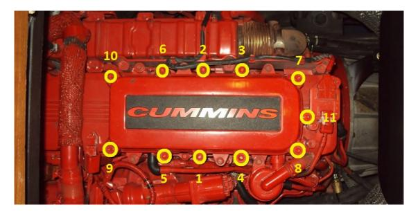
The final torque value for each bolt is **44 inch pounds**, starting at bolt 1 and working clockwise thru the 11 bolts as shown in the photo.
