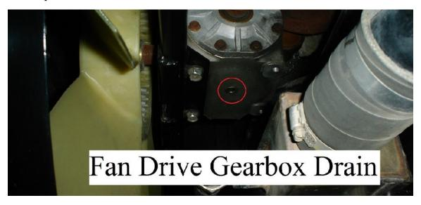
After the old lube had been allowed to completely drain the 3/8" plug was reinstalled. The engine access cover was removed to gain access to the 3/8" plug on the top of the gearbox where 24 ounces of new Shell Spirex 75W90 synthetic lube were poured in using the below funnel with a long flexible tube.
