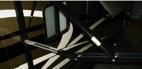
The left awning arm has an air spring built into the lower arm this allows that arm to collapse/lower in order to dump water from the accumulating on the patio awning.
