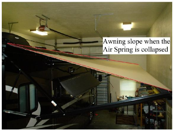
It is easy to see the difference in the awnings angle between the first photo and the last photo. The above photo shows the big slope difference between the front and rear edges of the patio awning. I do not know how many gallons or how much weight in pounds of water is required to activate the dump feature.
