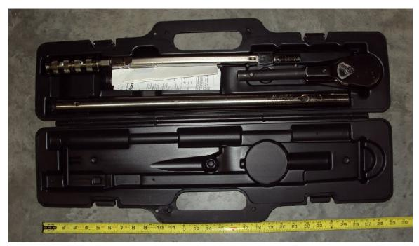
The case easily carries the three disassembled pieces of the torque wrench. Those three pieces snap together and the lug nuts 33MM 1" drive socket snaps on the 1 inch drive with a spring loaded pin to prevent the socket detaching from the wrench. Overall assembled length of the wrench is a shade under 48 inches and around 17 pounds.
