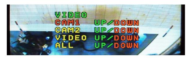
This menu allows the user to rotate any one or all camera images 180 ° (upside down) again by using the **CAMERA** and **VOLUME** buttons.
