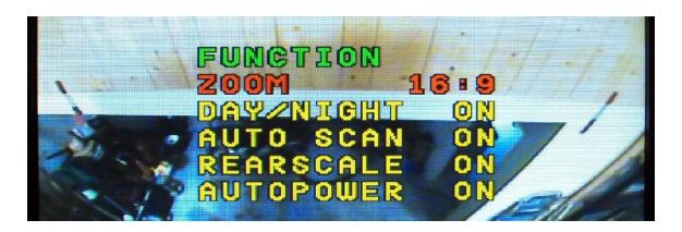
This photo shows the second menu, to get to this **FUNCTION** menu the **MENU** button is depressed <u>ONE MORE TIME</u>. Again as with the **PICTURE** menu the **CAMERA** button is used to select the row to change and the **VOLUME** buttons are used to make a change to **ON** or **OFF**, except for the **ZOOM** menu item which selects either a 4:3 or 16:9 screen.
