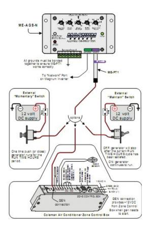
As seen above this option also contains a couple of other wiring options, those options control of the length of time the generator will run after receiving the generator start signal.
