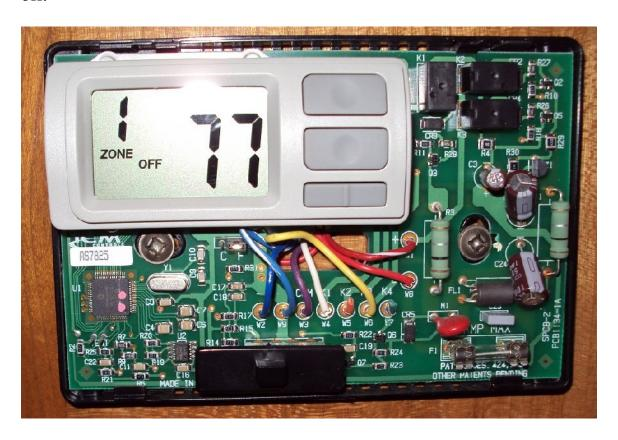
**Thermostat Communications**; the thermostat is connected to the following components, the coach fuse panel to power the thermostat, the Aqua-Hot and the three AC-HP control panels to signal there is a demand for heating or cooling.
