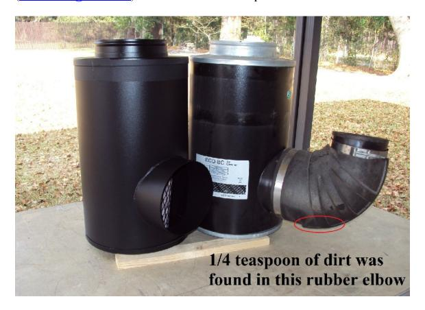
I did contact them about purchasing a filter, after reading the K& N air filter information we found the correct K & N air filter did not require oil, rather than a cotton filter it is a durable synthetic air filter media, according to the enclosed shipping information the filter is good for three years or 300,000 miles, however I also found written instructions stating the filter should be cleaned annually. The K & N filter requires a special cleaner @ \$22.00 per gallon, with free shipping.
