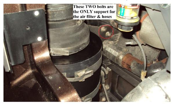
Other than the intake air hose and the output tubing to the turbocharger the two above bolts are the total support for the air filter and its metal mounting bracket. The metal at that point flexes allowing the air filter to move side to side not much but enough it could make a bumping noise.
