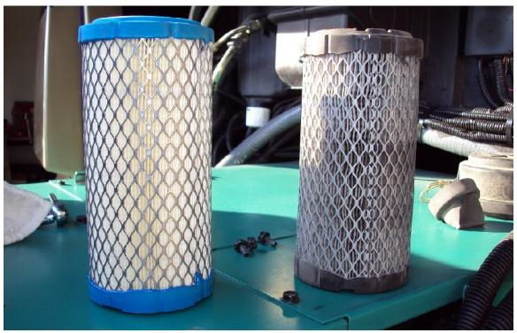
As seen in the above photo there was a significant amount of dirt based on the color difference in the old and new filters.
