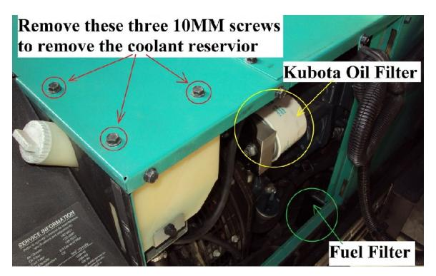
With the service panel removed the three filters are easily seen, however there is a few tricks to make servicing the filters easier.
