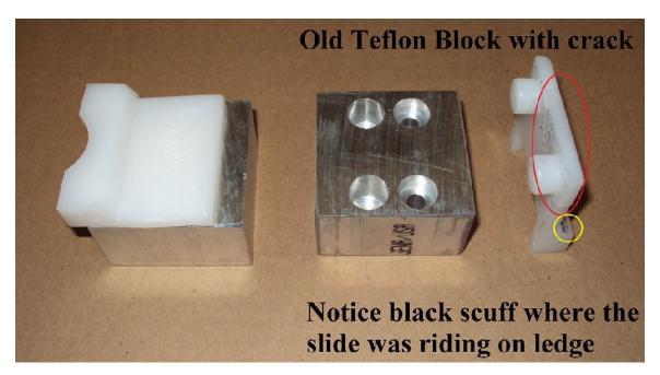
Replacing the broken block does not require many tools or a lot of effort. Two boards and a jack were used to lift the slide a couple of inches allowing the Teflon block to be removed and the new Teflon block to be inserted.
