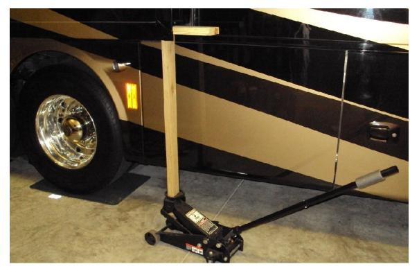
After inserting the block it's just a matter of slowly lowering the jack while making sure the slide is centered between the outside ledges on the Teflon blocks before completely lowering the slide. Based on the black scuff on the broken block there may be a need to move this aluminum block to the right another <sup>1</sup>/<sub>4</sub> inch, to prevent damaging another Teflon block, time will tell.
