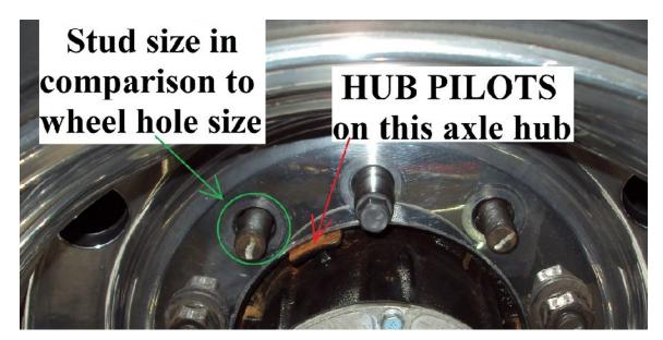
One method to prevent the occurrence of wheel and hub being assembled OFF-CENTER is to use a tool which actually centers the wheel on the wheel studs and not on the hub.
