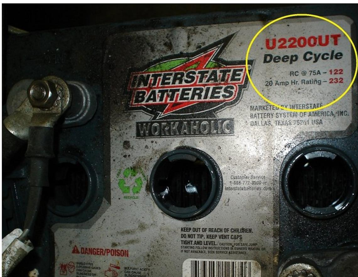
Notice the battery name and 20 Amp Hr. rating in the yellow circle. The 20 Amp Hr. rating was 232 Amp Hrs. on the U2200UT battery. When our HOUSE batteries were replaced in late February 2011 they were replaced with the new design Interstate GC2-HD-UT batteries, the U2200 batteries were no longer being sold, new batteries purchased by Tiffin on 2/3/2011.
