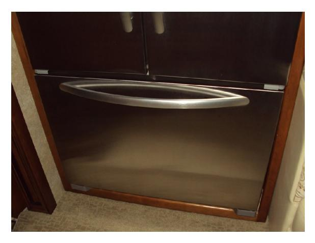
After seating the freezer handle over the tapered anchor the 1/8" Allen set screw was retightened. Since the Allen wrench was in hand all of the other Allen set screws on the door handles were checked before putting away the tools.
