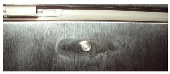
The above photo was taken after removing a 1/8" Allen set screw from the under-side of the freezer handle and swinging the handle out of the way. Next the screw was securely tightened and the handle was moved back into position ready to be seated over the tapered anchor as seen in the next photo.
