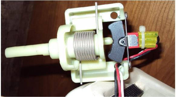
When you get to this point cut the white zip tie, remove the two switch screws remove the three slip on connectors from the three switch terminals. Plug the three slip on connectors on the new switch, reinstall the two switch screws, the three screws which hold the flush/dump mechanism in place and reinstall the lever. Install the cover if you are lucky to have a removable cover such as this one in our coach.
