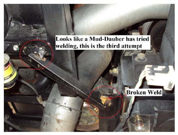
Removed the existing metal angle using an angle grinder, cleaned the metal surface to remove the welded material from the adjacent box steel and steel angle. Two 1/2" holes were drilled for installing bolts thru two locations on the box steel a third 1/2" hole was drilled in the coolant reservoir side brace. A piece of 1/4" thick by 2" wide steel flat bar was used to bridge the gap where the Tiffin installed support brace had been welded.
