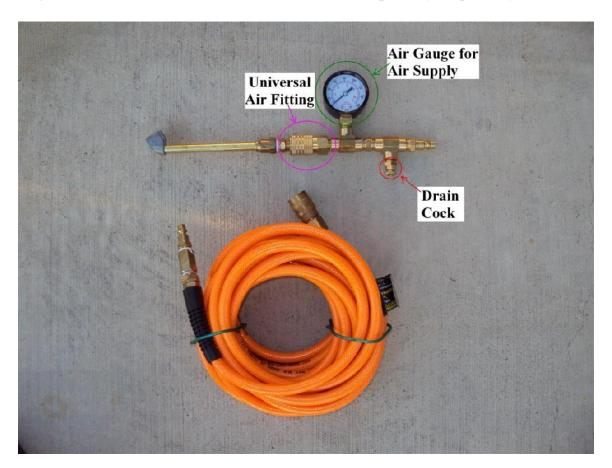
A couple of 25 foot coiled air hoses are carried which can be connected between to universal air fitting and the dual foot air chuck to provide more versatility.
