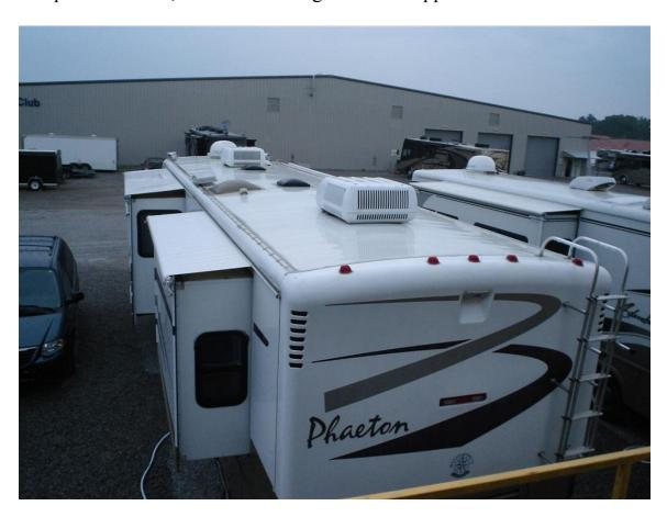
I believe during the 2007 model year Tiffin began using full sized roof panels which were manufactured with both cap rails as part of the complete fiberglass roof panel. The panels were all manufactured longer than needed for each specific model rolling down the line. If the coach was going to be a
