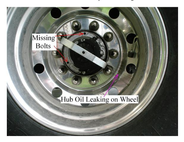
Notice two hub bolts are missing! They were completely missing they were not even contained inside the wheel hub. Makes me wonder about things?
