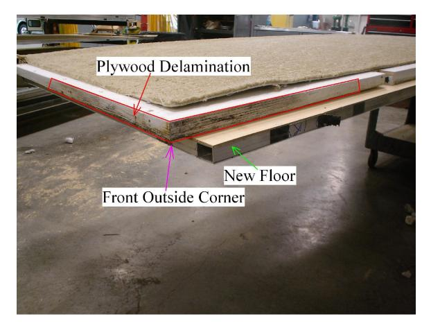
In the photo above the old delaminated floor is sitting on top of the new aluminum framed slide floor. The new floor weighs about one half the weight of the solid plywood floor it replaces.
