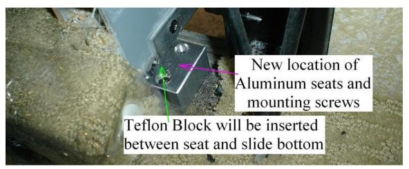
During this corrective work at Red Bay, three other coaches found one or both slide blocks broken on their bedroom slide? How are your slide blocks?
