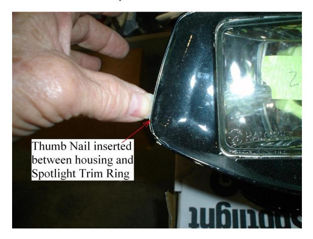
At the bottom of the housing near the trim ring is a single bump which locks the trim ring in place at the bottom of the housing. While on the top of the housing are two similar bumps. By carefully inserting a flat blade into the seam between the trim ring and the housing the ring can be separated from the housing.
