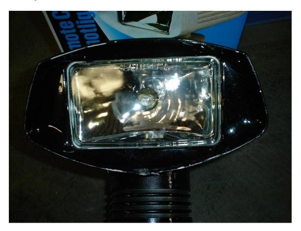
This Guest Remote Control Spotlight Model number 22200 uses a 50 watt Halogen bulb with a 100,000 candlepower beam, the bulb part number is 22230. This spotlight is also known by the name, Guest M-100 Spotlight. The whole secret is the knowledge of where the trim ring seam is located under that layer of paint.
