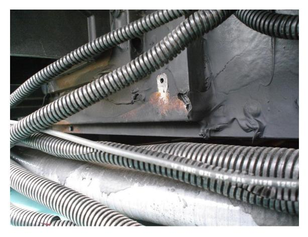
I understand some wiring is installed in the welding shop prior to the chassis being painted. But you can see in the above firewall photograph MOST of this wiring had been installed BEFORE the chassis had been undercoated or painted. The lower section of the firewall just above the generator had not been painted from side to side, also the bottom of the firewall had not been
