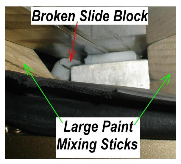
The above photo is the gliding block located on the left side of the passenger side bedroom slide. The broken block is easily seen with the rubber gasket pushed/pulled out of the way using the paint mixing sticks.
