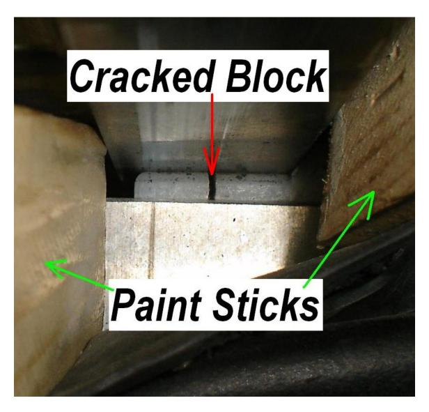
The above photo is the right side of the passenger bedroom slide the block is cracked in two pieces. This is just another item one of many for Tiffin to correct.
