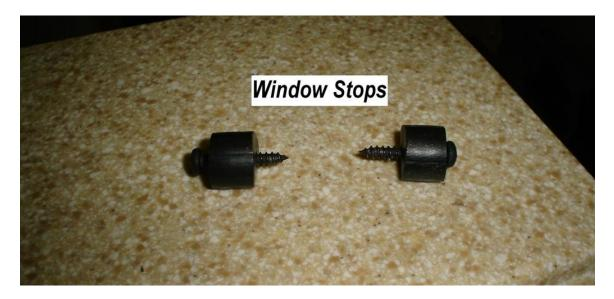
As seen in the below photo the window can be raised enough with the two rubber stops removed to allow accessing the entire inside of the slide window for cleaning.
