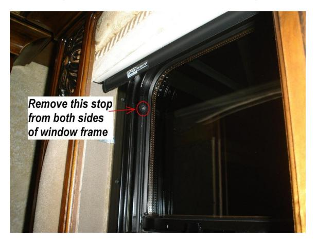
The window clip used to hold the window open is mounted on the right side of the frame. The window clip must be held back so the window can be raised past and above the clip.
