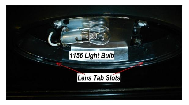
Reinstalling the lens is not hard to do just insert the bottom tab(s) then apply gentle pressure on the top of the lens until the lens snaps into place.
