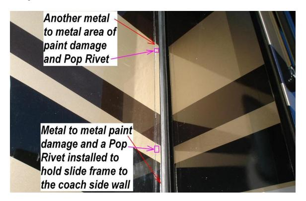
After the pop rivets had been installed the coach was sent to the body shop to have the damaged area sanded, prepped, painted and caulked.
