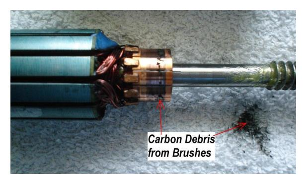
After motor housing disassembly the carbon on both the copper commutator and the towel are both evident.
